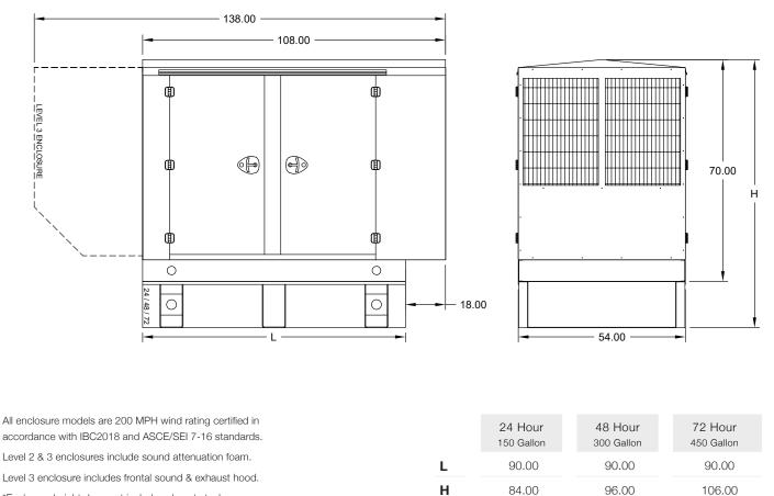
\*Enclosure height does not include exhaust stack.
